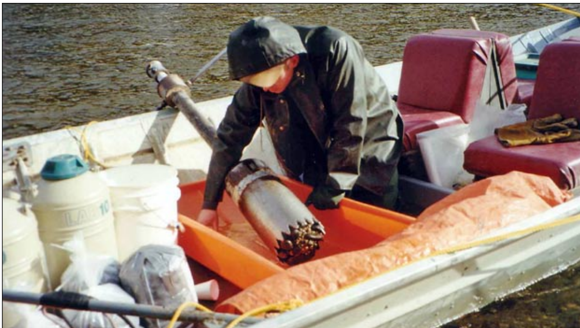
Freeze core sampler pulled from substrate and lifted onboard a boat for sample extraction
